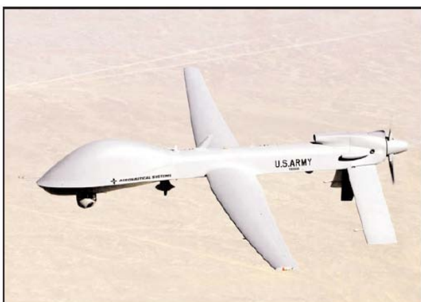
General Atomics Aeronautical Systems' Warrior unmanned aerial vehicle. Photo courtesy General Atomics.
