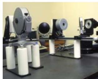
Sira's modulation transfer function test equipment. Image credit: SSTL
