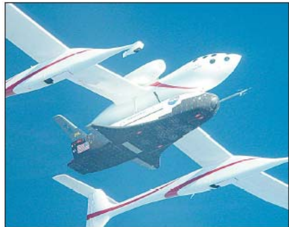
The White Knight carries the X-37 beneath its fuselage.
