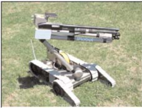
iRobot has developed a PackBot prototype armed with a shotgun. Photo courtesy iRobot.
