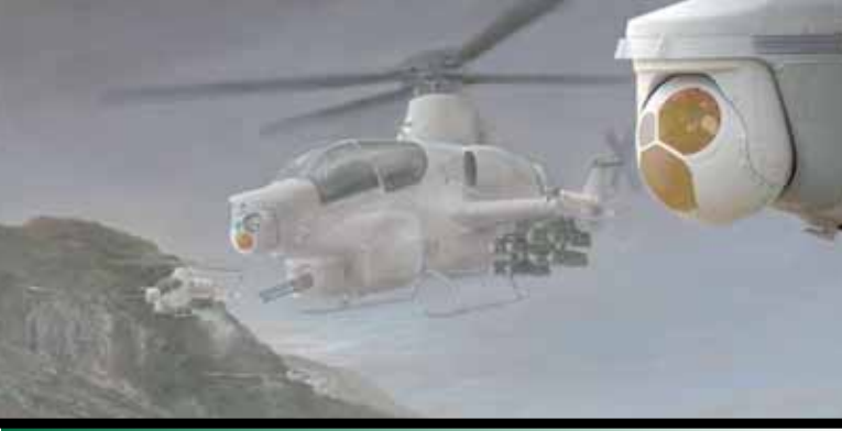
Target Sight System (TSS) Electro-Optical/Infrared Targeting System for the US Marine Corps AH-1Z
