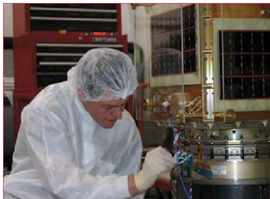
Figure 4. Cadets, working with lab technicians, carefully integrate the many parts of FalconSAT-3, to include the Lightband, a mechanism that will release the satellite from the launch vehicle payload adapter into its final orbit.
