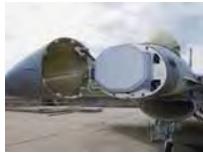
Raytheon has demonstrated RACR s physical compatibility with the F-16 via the installation of the form-fit model shown here (Raytheon)
