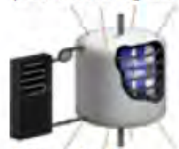
Propulsion & Cryogenics: Zero boil off cryogenic propellant storage to enable long duration missions
