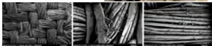
Electron micrographs from GRC showing damage to the outer layer of Alan Bean's Apollo 12 suit
