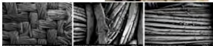
Electron micrographs from GRC showing damage to the outer layer of Alan Bean's Apollo 12 suit
