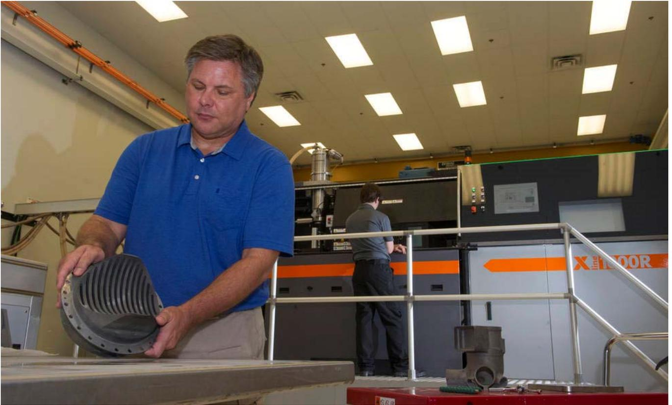
Andy Hardin, a subsystems manager in Marshall's Liquid Engines Office, inspects a 3-D printed rocket part made with a selective-laser-melting machine in the Advanced Manufacturing Lab.
