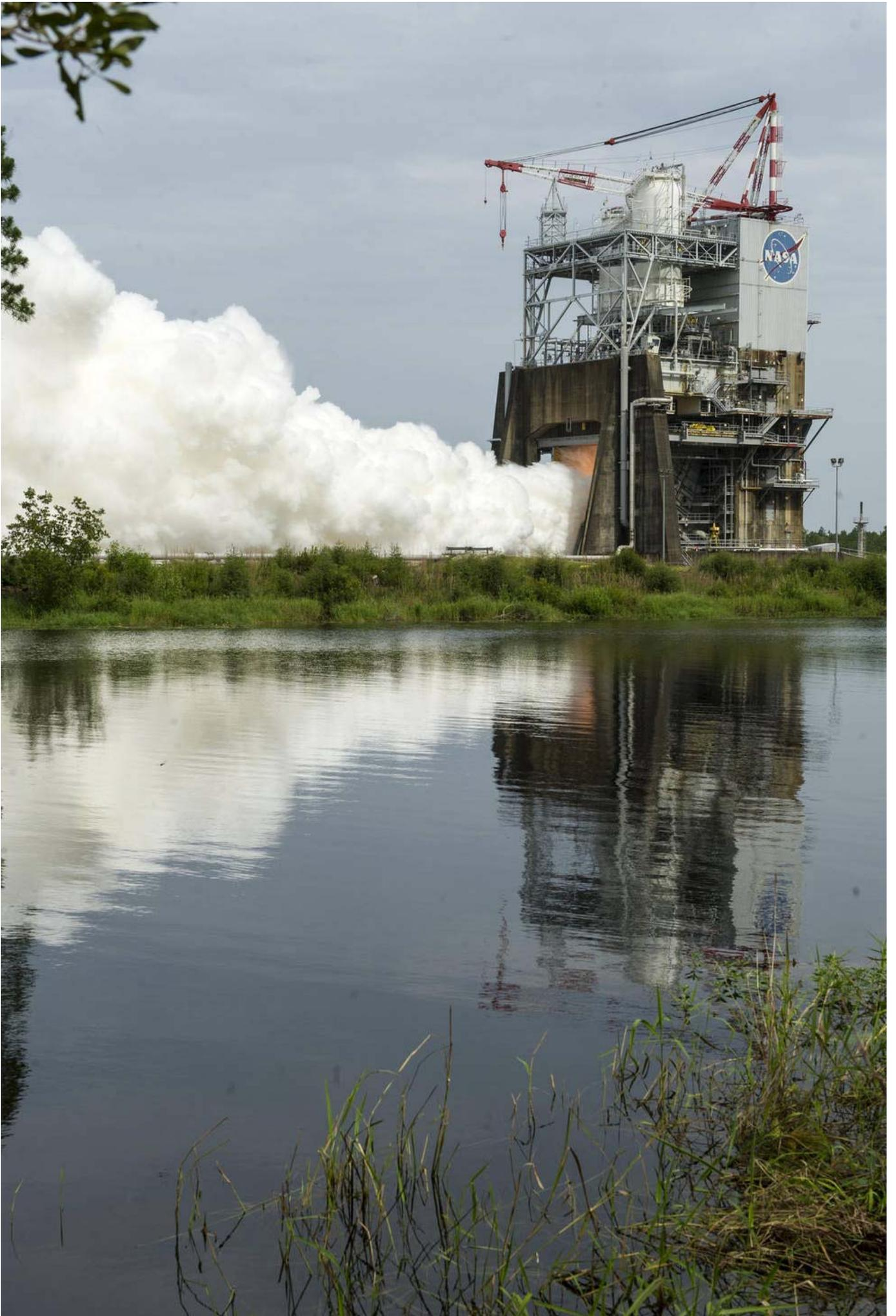
On June 25, engineers at NASA's Stennis Space Center conducted a 650-second test of a RS-25 developmental engine. Four RS-25 engines will power the core stage of NASA's new rocket, the Space Launch System, on deep-space missions, including to an asteroid and ultimately to Mars. Three additional tests are scheduled this summer before the initial series is complete. See more information on the test [here](#).
