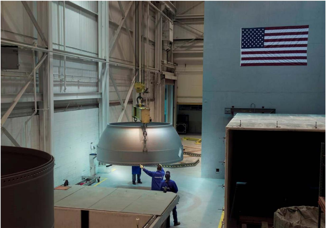
Technicians at Orbital ATK offload the aft dome that will be used on one of the two, five-segment [solid rocket boosters](#) for the first flight of SLS. Like the aft stiffener, the aft dome is a component of the aft segment of the booster. NASA's Marshall Space Flight Center manages the SLS Program for the agency. (Orbital ATK)
