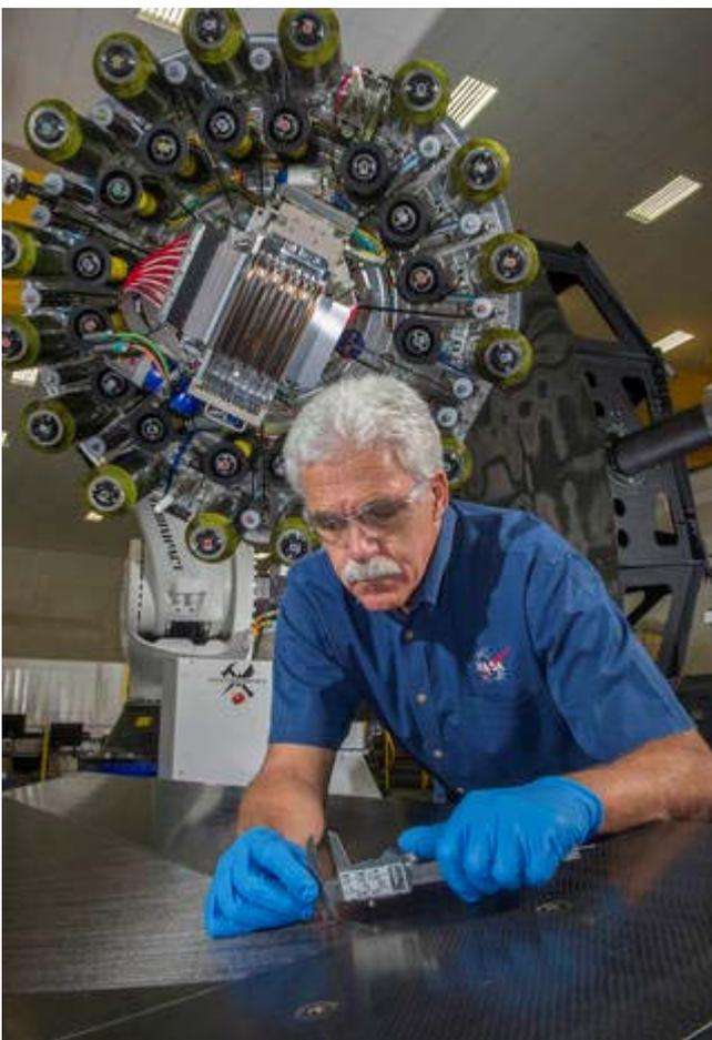
Larry Pelham, a materials engineer in Marshall's Composites Technology Center, checks the spacing between carbon fiber layers during a test-build by the new robot. Behind him is the head of the device that spools out the fibers to create parts for new space vehicles.
